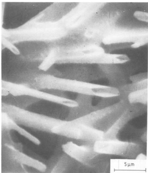
Figure 4 Scanning electron fractograph of heat treated, leached and then sintered at 1580°C for 5 min, Sample 3. Strong crystallization present.
