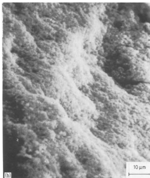
Figure 3 Scanning electron fractograph of heat treated and then leached samples: (a) Sample 2 (b) Sample 3.
